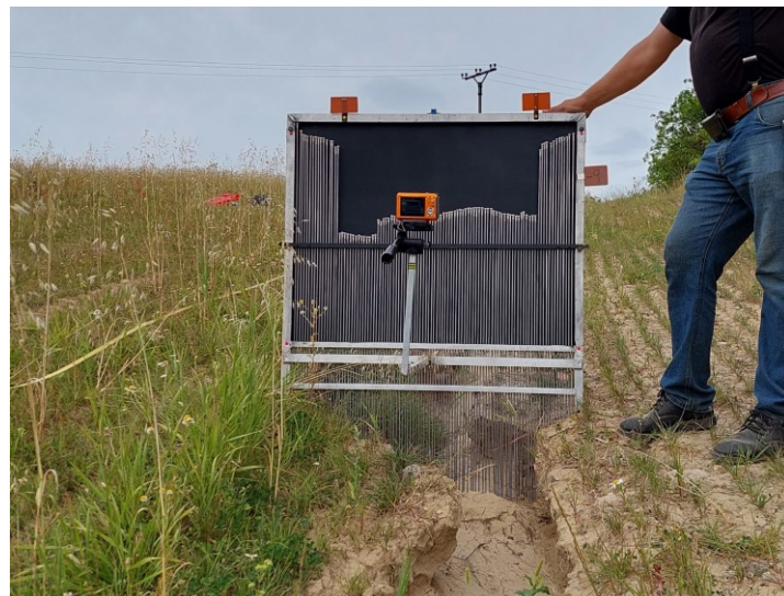
Fig. 4 Measuring with the use of the erosion bridge and its main parts [own source]
